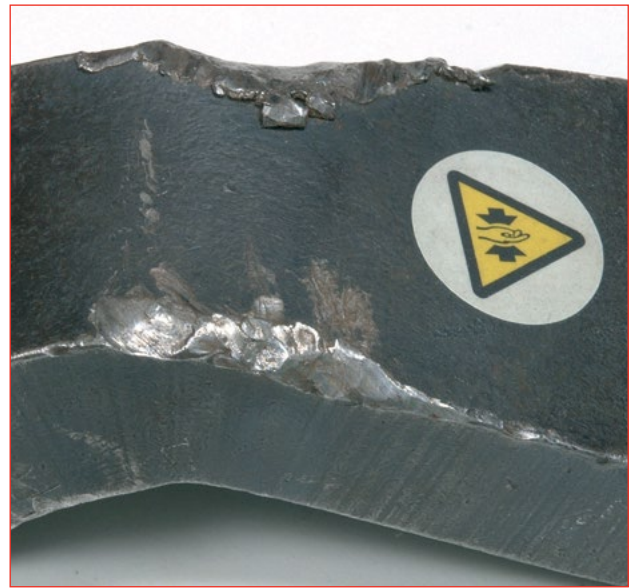
Signs of poor reaction are evident on this damaged foot. Reaction was taken at the wrong point on the foot and burring indicates that the foot was slipping off the reaction point.
