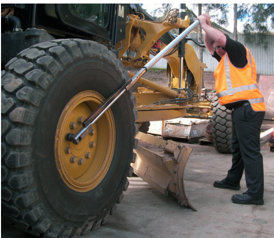
Without a torque multiplier
