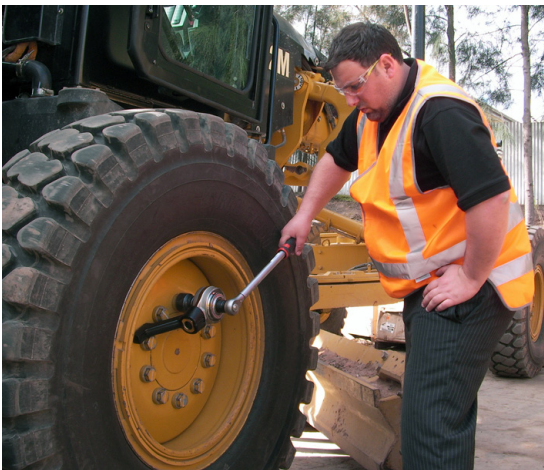
With a torque multiplier
